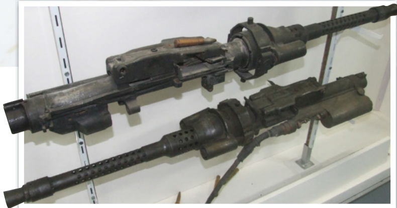
Below: The Rheinmetall MG 131 13mm heavy machine gun was designed for use in several types of mounts aboard Luftwaffe aircraft
